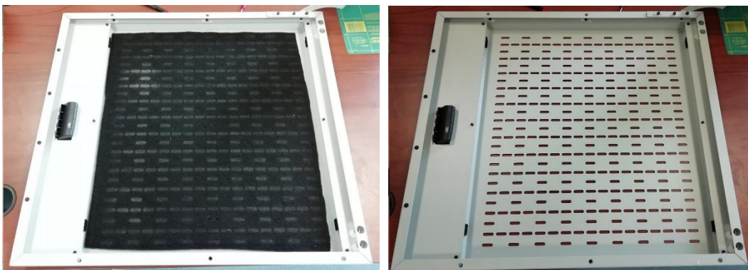
Fig. 14 Removing the used filter
