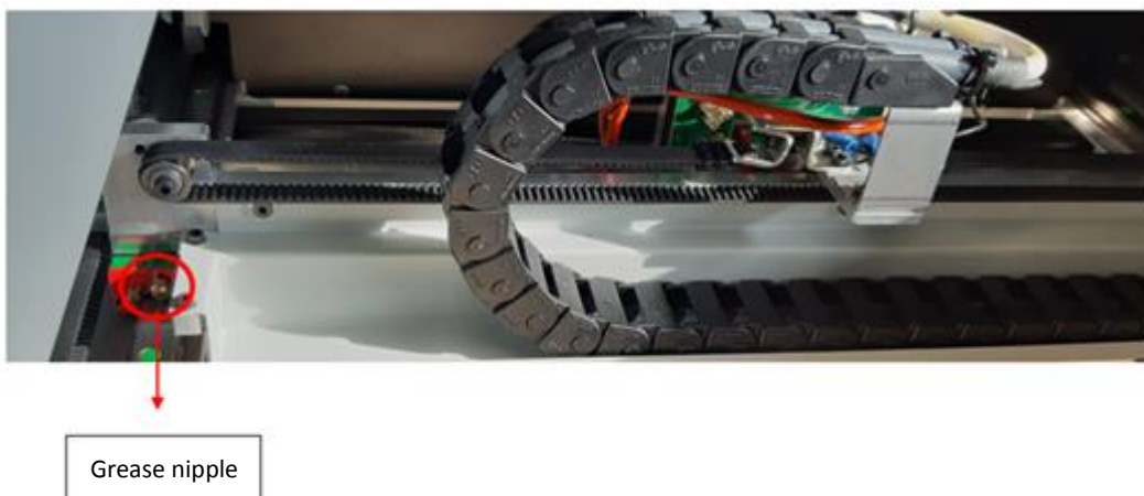
Fig. 31 Lubricating the front linear carriage of the X axis
