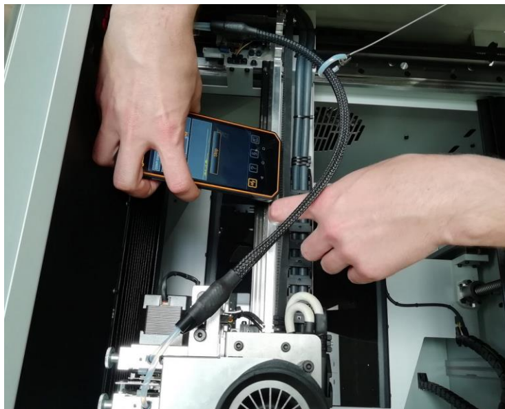
Fig. 45 Measurement location of the timing belt tension on the Y axis
