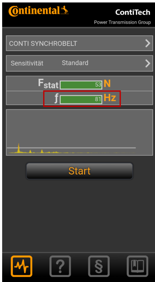
Fig. 43 Measured value of toothed belt tension
