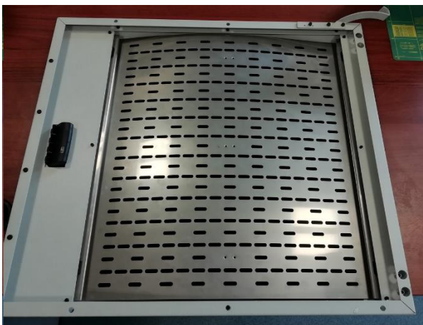
Fig. 12 Reversing the top cover
