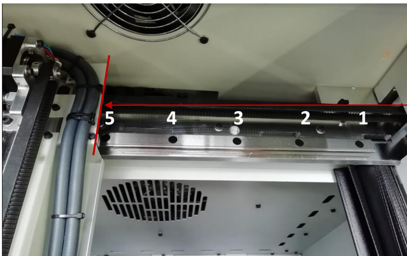
Fig. 39 Setting up the X axis carriage
