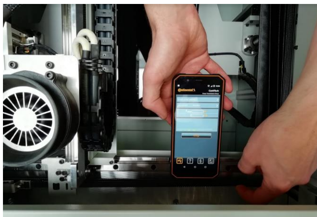
Fig. 44 Measurement location of timing belt tension on the X2 axis
